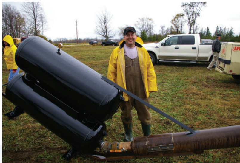
Kent Cruickshank and his cannon, "Rusty Brown." At Kent's feet is the yellow trigger valve and the hatch in the barrel where the pumpkin is loaded.
